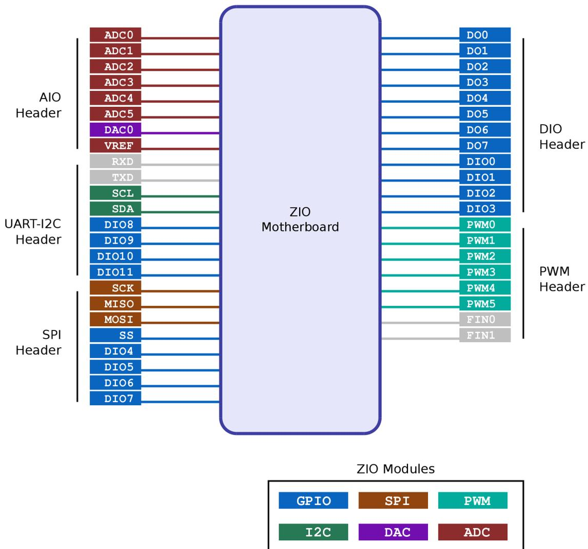
These modules on the motherboard are accessed through an agent software running on the motherboard. The API communicates with the agent and performs actions on the modules. Each module is handled by a separate object class in the API. The modules and their corresponding classes are described in detail in the following sections.
